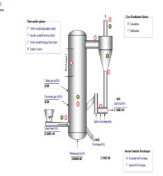
The figure above represents the main CFB design window. A number of options being accessible directly on the work sheet the choice of flow model and the discharge evaluation.
