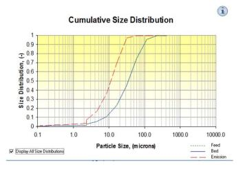
The above graph exhibits the cumulative size distribution in the dryer. It is for size distribution at bed, grid and cyclone emission.
