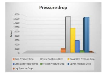
The above Bar graph represents the pressure drop in all the components and aspects of fluidized bed dryer.
