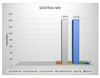
The above Bar graph represents the solid flow rate in the components of circulating fluidized bed dryer. The rate of flow is referred in tonnes/hour.
