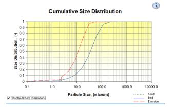
The above graph presents cumulative size distribution at solid feed in the CFB here it is clearly showing the feed and bed have particle size more than the emission.
